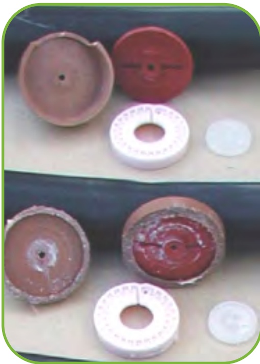
Figure 43. Self compensating drippers (2 litre/h) with Ultrasol™ Magnum P44 (200 ppm P_2O_5 ) at top and MAP (200 ppm P_2O_5 ) at bottom.
