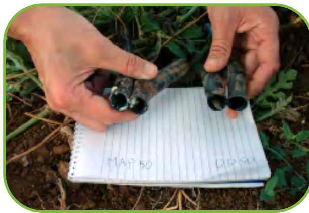
Figure 42. Drip lines of a fertigation system in a tomato field trial in Crete, Greece (2002): The lines on the left had been constantly supplied with MAP, on the right with Ultrasol™ Magnum P44 over the trial period. All other treatments remained the same. The higher amounts of precipitates in the MAP treated lines is obvious.
