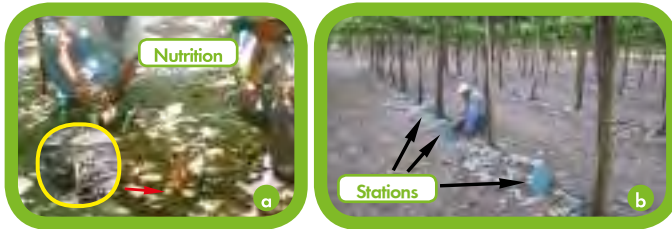
Figure 26. Nutritional Monitoring, using probes or porous capsule extractometers of different types: left picture (a) shows two types of extractometers: the one of a larger diameter (white) corresponds to the Spanish exclusive extractometer distributed by Agriquem Chile S. A.; the one marked with a yellow circle is of Israeli origin, which is similar to a tensiometer but carries a hose for suctioning the solution. Picture (b) depicts four measurement stations at different depths: 30, 60, 90 and 120 cm (Israeli system) (Palma, 2004. Field visit, SQMC Chile).
