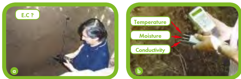
Figure 24. Monitoring electrical conductivity (a), and moisture and temperature testing (b) (Palma, 2003. Technical Assistance SQMC, Chile; Callejas, 2004, field visits. Copiapo, Chile).
