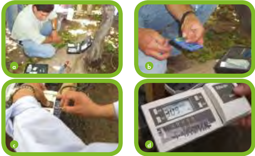
Figure 28. Nutritional monitoring with extractometer with an electrode equipment (Habira brand (a and b), Cardy), and irrigation bulb by means of measurable saturation extract with a Reflectoquant RQ-Flex Plus (Merck) (Palma, 2003. Field visit, Chile and Colombia).
